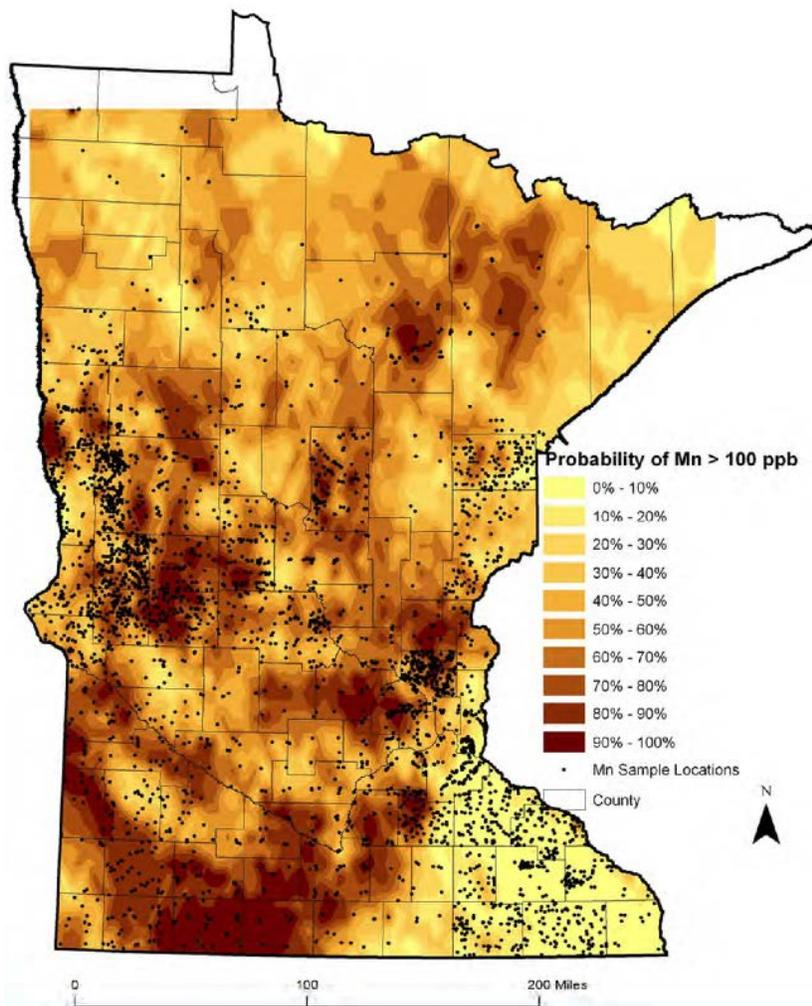
Figure 2: Probability of Manganese Greater than 100  $\mu\text{g/L}$  in Minnesota Groundwater<sup>8</sup>
