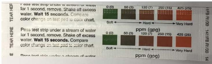
Figure 15: Hach Water Hardness Test Strip
