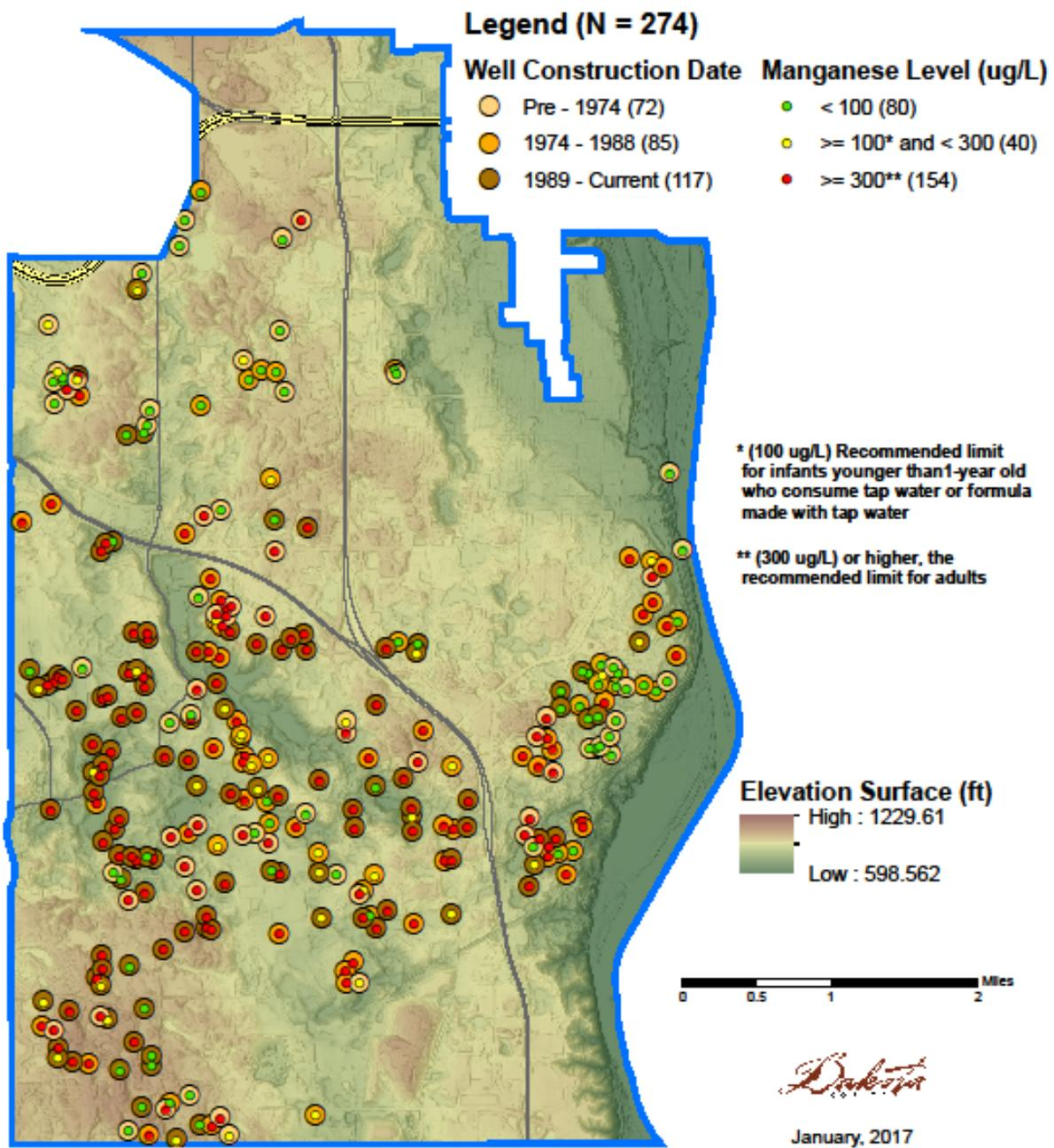
Figure 29: Manganese concentration by well construction date
